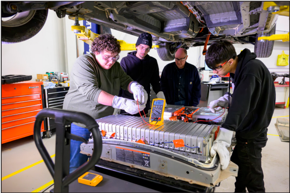
Moraine Valley Community College Automotive Technology students, under the instruction of adjunct professor Steve Tyrolt, remove an EV battery.
